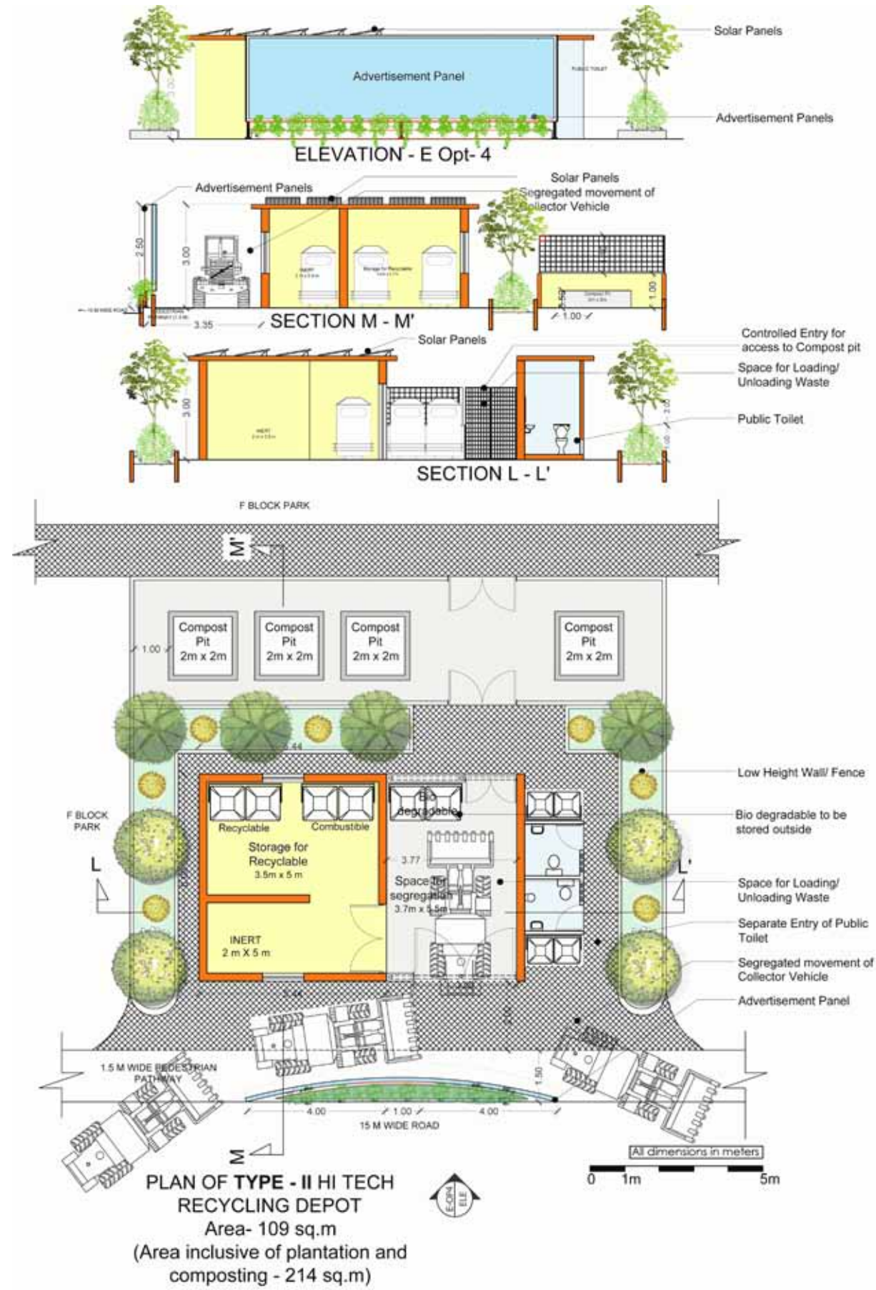
Hi Tech Recycling Depot: Type II – Option 3 – Plan, Sections and Elevation
