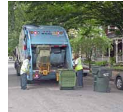
Colour coded bins (Door-to-door) collection Source: http://www.richmondgov.com/PublicWorks/RefuseCollection.aspx
