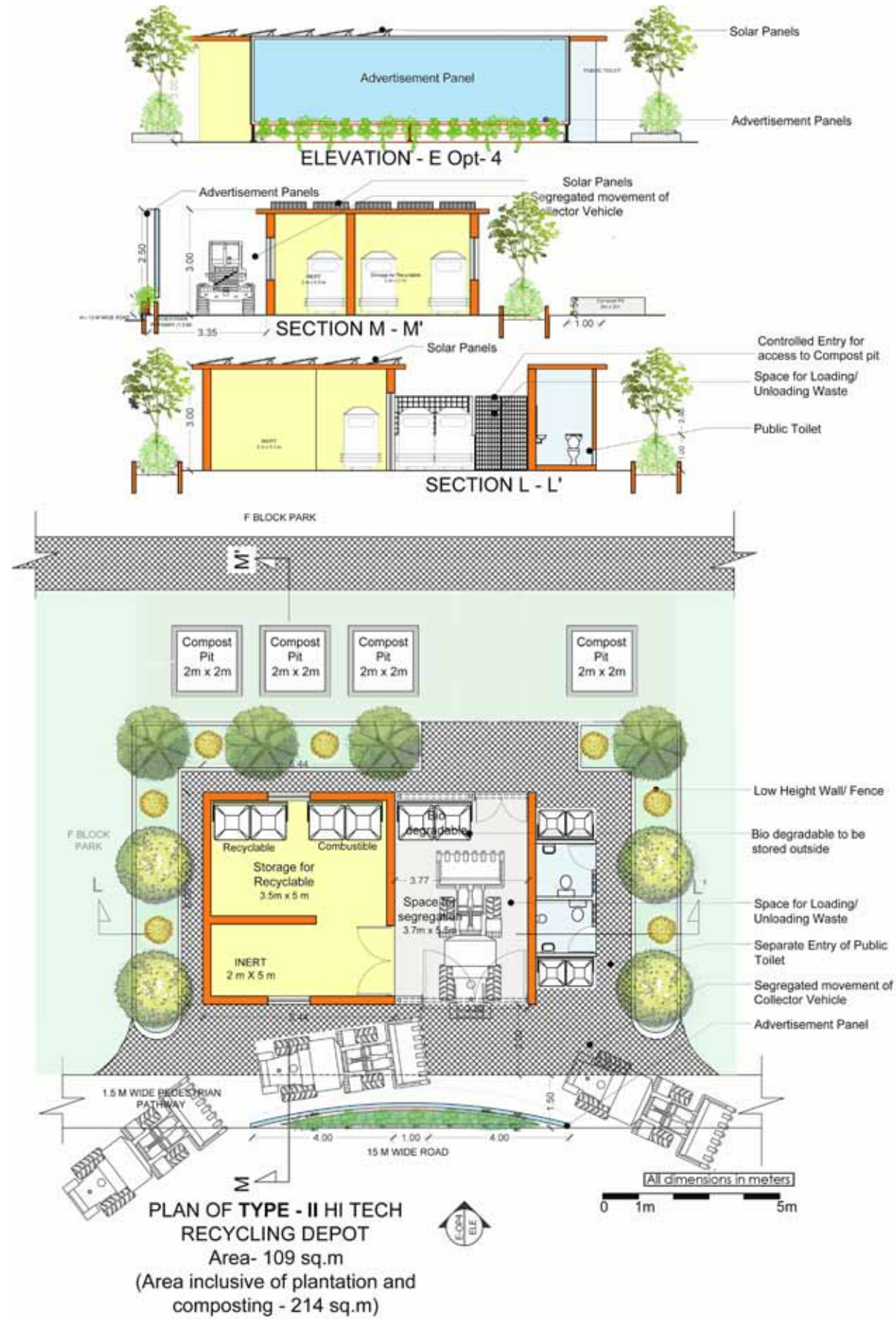
Hi Tech Recycling Depot: Type II – Option 4 – Plan, Sections and Elevation
